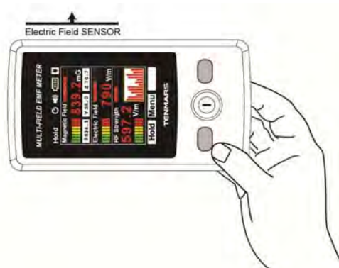
Figure 3 – Orienting the meter for Electrical Field Measurements
